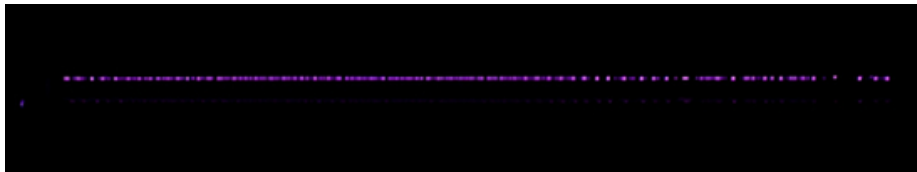
Figure 1-4: Negative corona discharge
